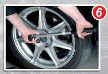
6. The correct torque Tighten all wheels to the specified torque.
