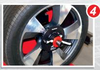
**4. On the balancing machine** Observe the correct clamping of the wheel on the balancing machine. The SoftGrip firmly clamps the wheel to the shaft.
