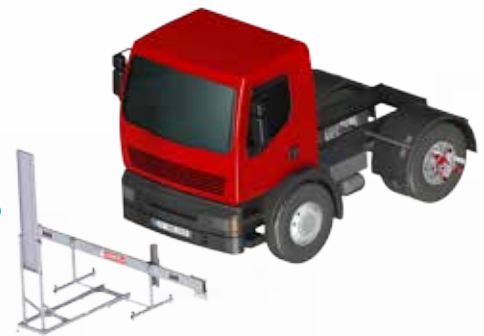
The measuring crosshead and calibration reflector are aligned horizontally at an exact distance in front of the vehicle.
