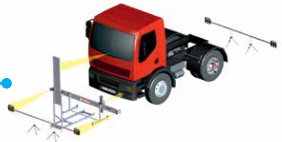
The measuring crosshead and calibration reflector are aligned horizontally at an exact distance in front of the vehicle.
