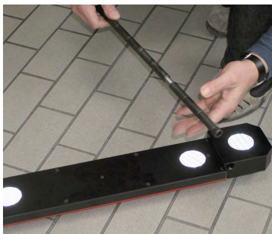
Unscrew the ends of the attachment bars.
