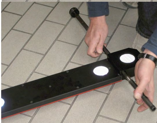
Guide the attachment bars through the scale and screw them back together.
