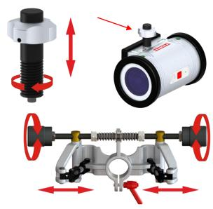
It must be possible to slightly rotate the spindle from the tensioning head in both directions. The swivel arms must not jam and they are kept in the middle in the same position by the spring force.
